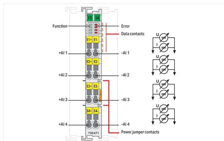
This analog input module processes both voltage and current differential signals.
